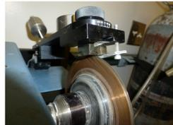
Fig. 1: Dicing Saw
